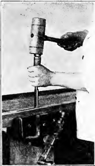
FIG. 261. LAST STEP IN MORTISING.
